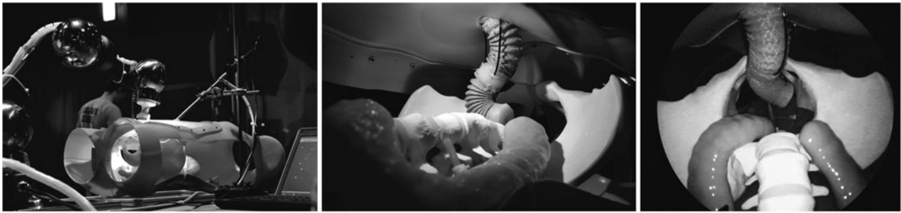
FIG. 5. The current version of the STIFF-FLOP manipulator with two independently controllable soft modules. On the left the overall platform is shown. The central and left images show the manipulator inside the phantom; the picture on the left is the view from a laparoscope.
