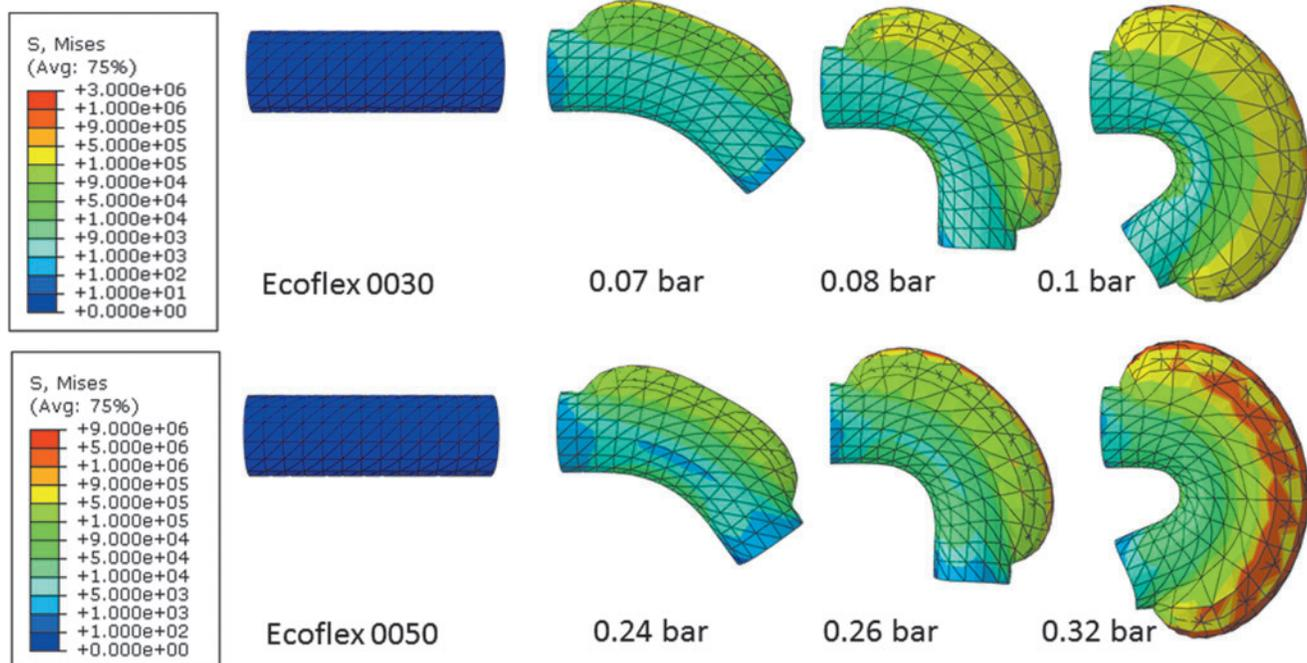
**FIG. 5.** FEA simulations of a module (with three semicircular pneumatic chambers, length=8 mm) actuated in one degree of freedom bending mode: comparison between Ecoflex 0030 and Ecoflex 0050 modules at different inputted actuating pressures to achieve the same bending angles in both types of modules. Color images available online at [www.liebertpub.com/soro](http://www.liebertpub.com/soro)
