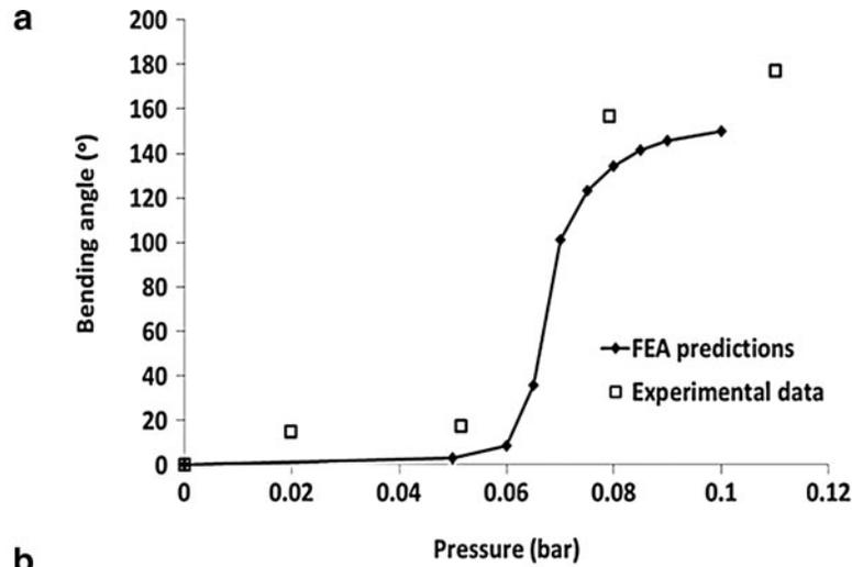
**FIG. 4.** Experiment versus finite element analysis (FEA) predictions of module bending under one-chamber actuation (a) FEA predictions and experimental data from the tip-tracking magnetic sensor of the bending angle at the tip of an Ecoflex 0030 module (three circular cross-sectional chambers, length = 8 mm). (b) Ecoflex 0030 module under one-chamber actuation at 0.1 bar. (c) Ecoflex 0050 module (three semicircular pneumatic chambers) under one-chamber actuation.
