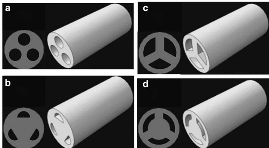
**FIG. 1.** Investigated pneumatic chamber designs for the pneumatic actuator module for a soft-arm medical surgical robot; module diameter is 25 mm; cross-section of the three pneumatic chambers: (a) circular cross-section; (b) semicircular cross-section; (c) circular sector cross-section; (d) ring sector cross-section.
