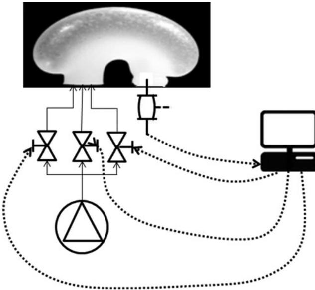
**FIG. 2.** Diagram of actuation and tip position track system for a silicone module with three pneumatic chambers.
