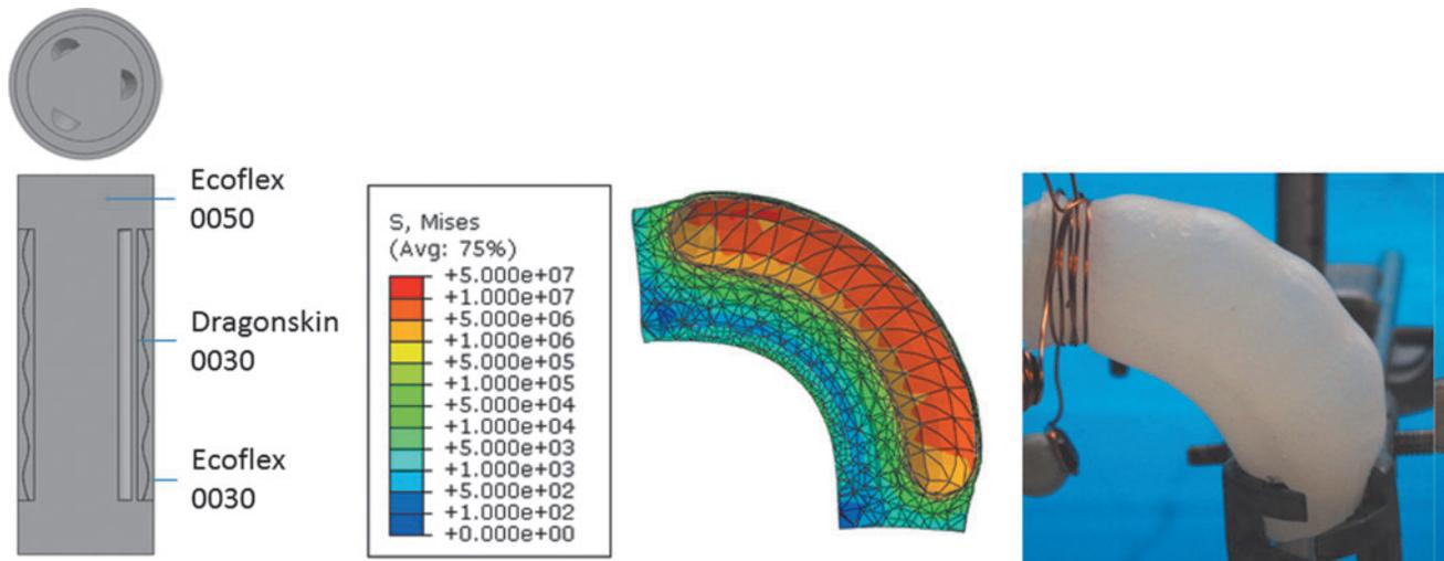
**FIG. 7.** Module with Dragonskin 0030 accordion structure: module design, FEA analysis, and experimental study of one-chamber actuation under 0.8 bar. Color images available online at [www.liebertpub.com/soro](http://www.liebertpub.com/soro)
