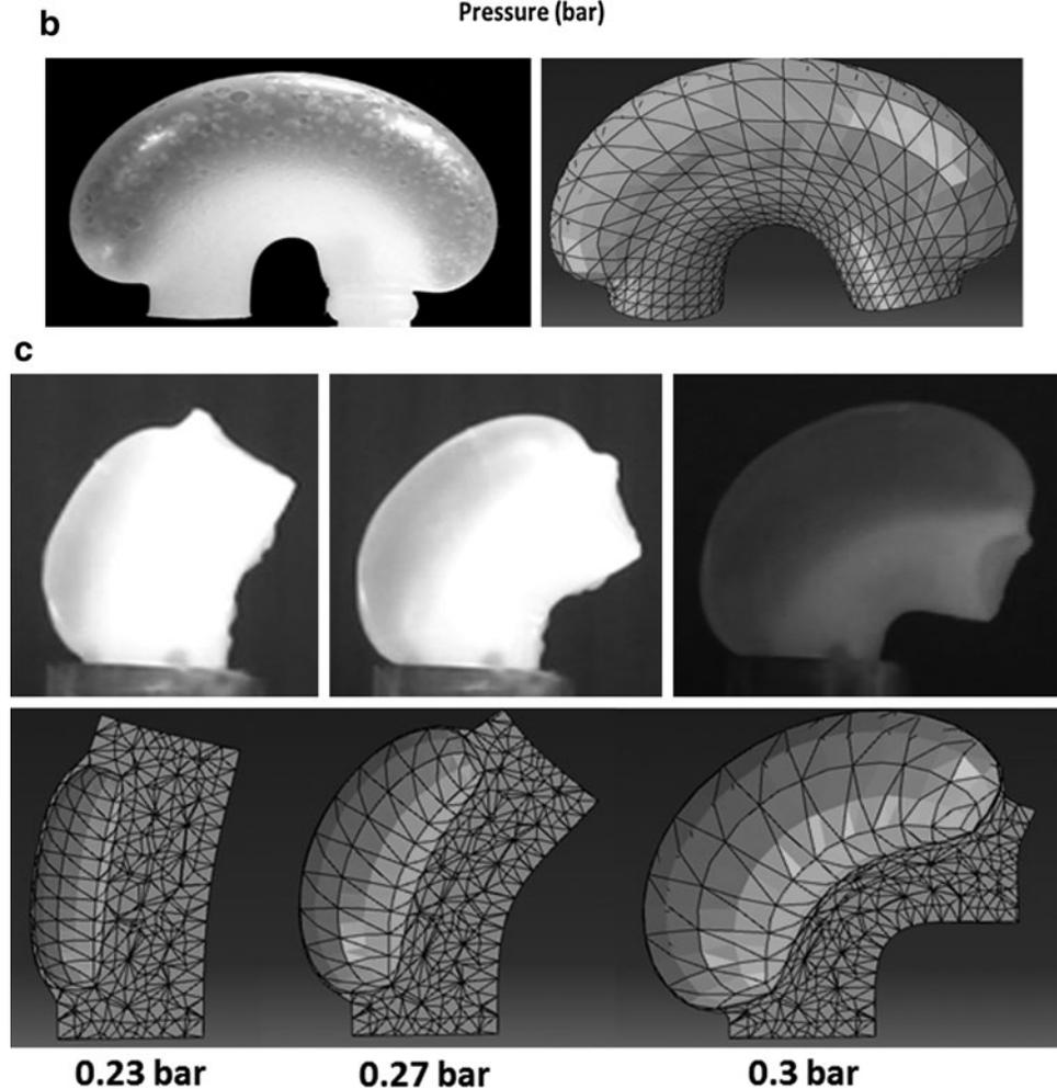
pneumatic chamber at 0.1 bar: using image analysis tools, the maximum radial width of the expanded silicone module (experimental) was measured to be 41.2 mm against the original 25 mm, whereas the FEA-predicted radial width was 40.7 mm at the same actuating pressure.
