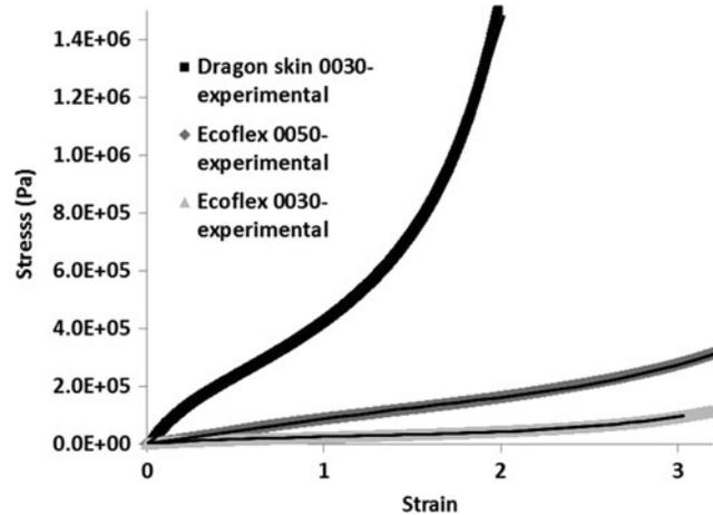
**FIG. 3.** Best constitutive model stress–strain lines against the corresponding experimental data: Yeoh constitutive model for Ecoflex 0030 and Ogden constitutive model ( $N=3$ ) for Ecoflex 0050 and second-order reduced polynomial for Dragonskin 0030.
