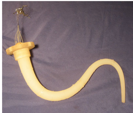
Fig. 1. Soft robot arm driven by 12 cables embedded inside the silicone body and fastened at different distance from the base. This is the prototype used for the experimental validation of the dynamic model presented in this paper.
