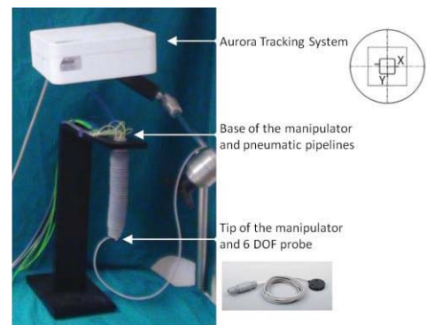
Fig. 3. Set up for the tracking of the tip position during manipulator motion.
