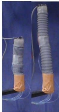
**Figure 13:** Left, 2-module manipulator not actuated. Right, fully elongated manipulator with 0.065 MPa the three chambers of each module.
