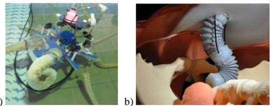
Fig. 1. The eight-arm OCTOPUS robot (a); the STIFF-FLOP surgical manipulator (b).
